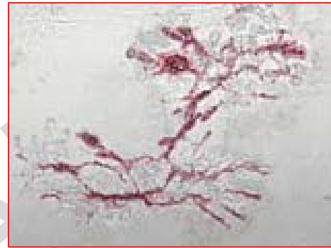
Liquid Penetrant (Penetrant bleed out)
