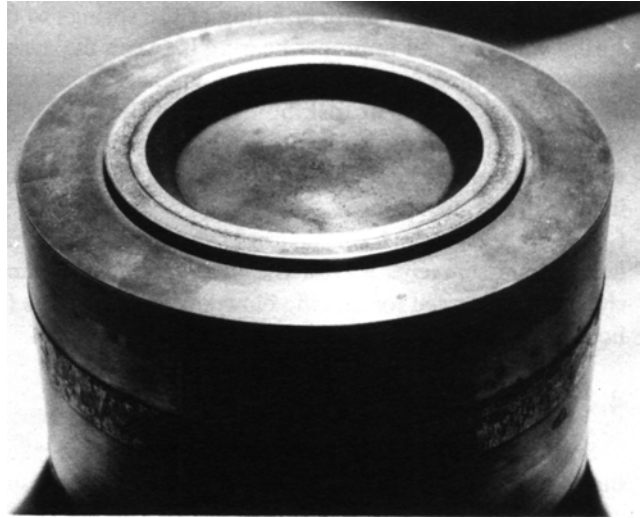
Figure 27—Seating Surface of Disk Deformed by Chattering
