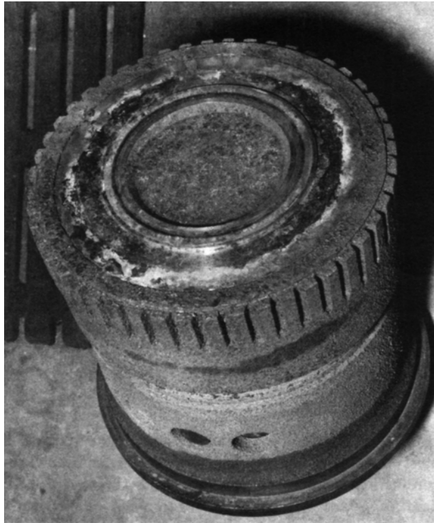
Figure 35—Disk Frozen in Guide Because of Buildup of Products of Corrosion in Sour Oil Vapor Service
