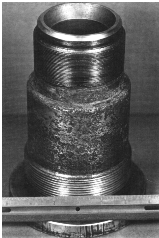
Figure 21—Chloride Corrosion on 18Cr-8Ni Steel Nozzle (with Machined Seating Surface)
