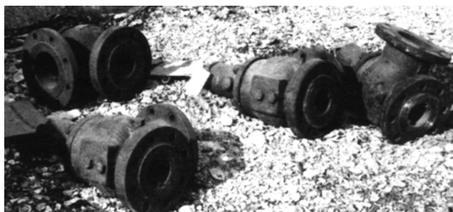
Figure 36—Rough Handling of Valves Should be Avoided
